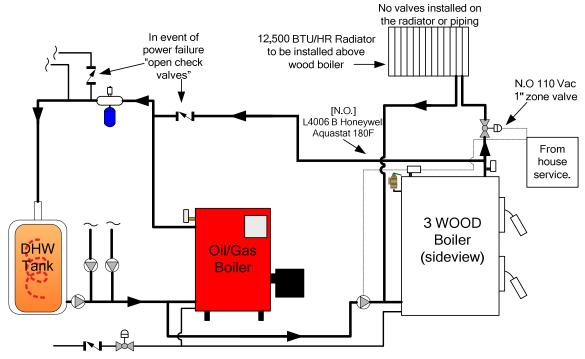
Should your electricity go off during the heating season, there are several procedures that should be followed in order that you may continue to safely operate your heating system. These procedures apply to the solid-fuel boiler, as the gas or oil-fired boiler, if any, will be completely inoperative.
