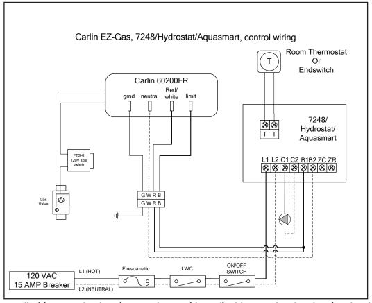
NOTE: All wiring must be done in accordance with applicable state, local and national codes. Use only copper conductors.
