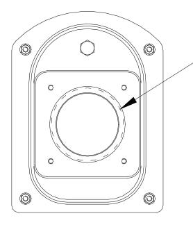
TRIM INSULATION IN BOILER DOOR OPENING TO 4.25" FOR BECKETT AFG AND CARLIN EZ BLAST TUBE.
